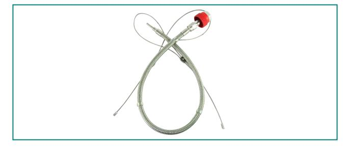
Pigtails in stainless steel 1.4404 are for connecting gas cylinders with gas supply panels. The pigtails are fitted with a hand nut and gas specific connections to DIN477 -1 or -5 (300 bar).
